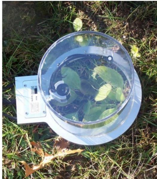
Figure 16: The CPY-4 transparent chamber used to measure efflux from low lying vegetation.
