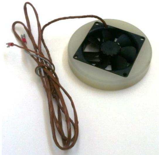
Figure 35: The electrical blowing fan with its side white cover. The fan is intended to be used for the dynamic chamber operational mode.
