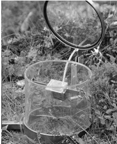
Figure 12: A small in height static chamber.
