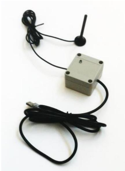
Figure 34: The wireless USB connection that will be connected to the laptop.
