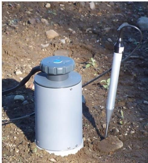
Figure 15: The PP Systems SRC-1 none transparent chamber model used to measure soil efflux.
